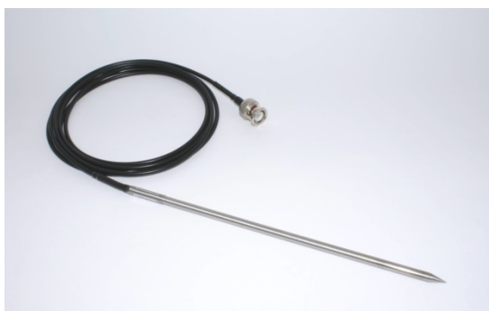
Fig. 21. LP/t - laboratory probe for soil temperature
